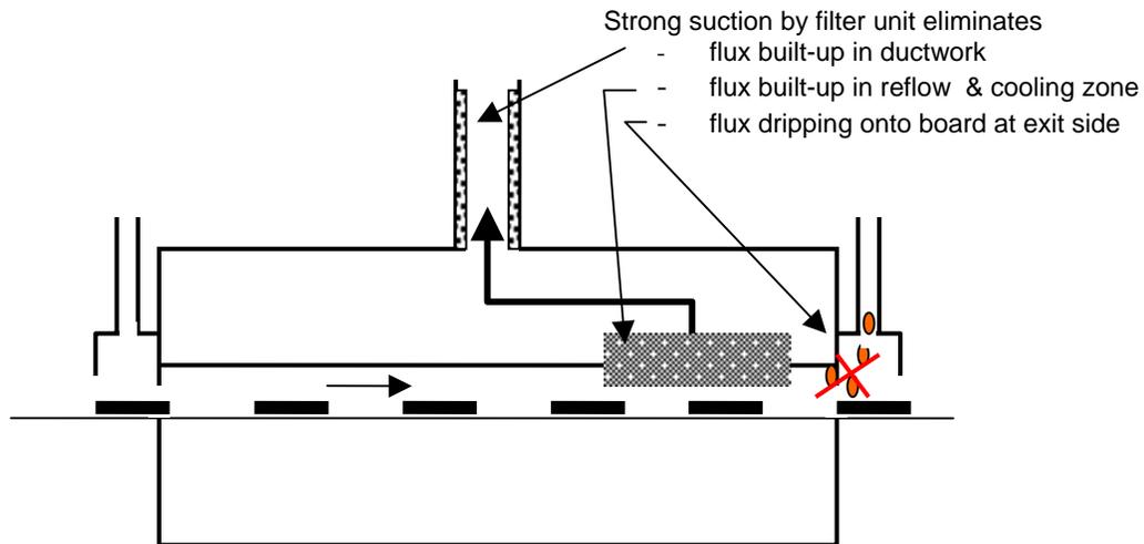
A dedicated filter unit provides more consistent airflow, enhances the process control and can reduce maintenance costs.
