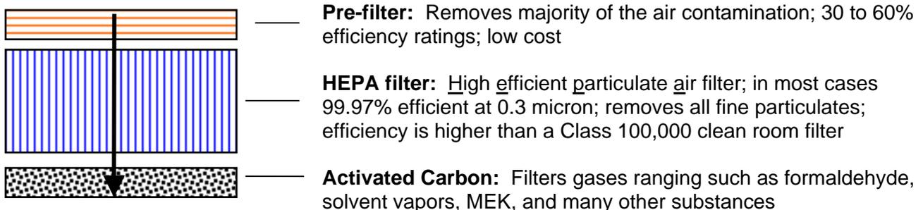
Optional **after-filters** can be supplied with the F8200 series. These filters further reduce the particle count in the exhaust which may be helpful in semi-cleanroom application conditions.
