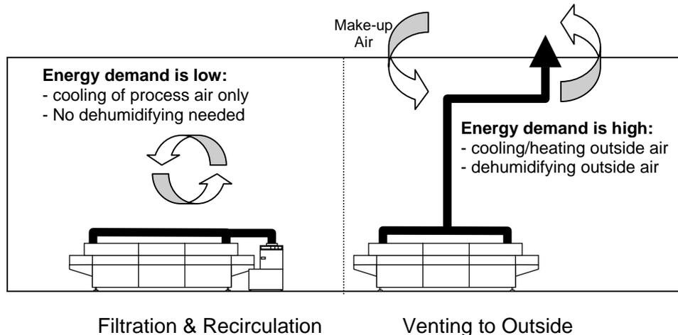
Any air vented to the outside of a facility has to be replaced with make-up air from the outside. When venting 1,000 cfm from a wave solder machine to the outside, the air conditioning system has to supply the plant with 1,000 cfm of “make-up air” to maintain the balance inside the building. Therefore, the energy or heat impact of filtration and recirculation is the difference between cooling process air from inside the facility or cooling/heating make-up air from outside.
