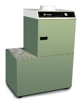
The F8230C and F8240C models are designed for the connection to production line equipment such as wave solder units and other applications requiring high airflow rates. Pre-filters and high capacity HEPA filters assure a long filter life. The unit features multiple filter status indicators, warning lights and a front access door for easy filter maintenance.
