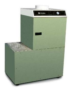
The F8220C filter unit is designed for the connection to production line equipment such as reflow or curing ovens and wave solder units. Large filter sizes allow for high airflow rates and assure a long filter life. The unit features multiple filter status indicators. warning lights and a front access door for easy filter maintenance.
